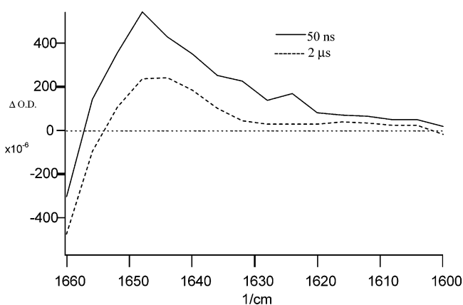
Figure 10. Transient IR spectrum produced upon LFP (266 nm) photolysis of 1F in dioxane at ambient temperature.
